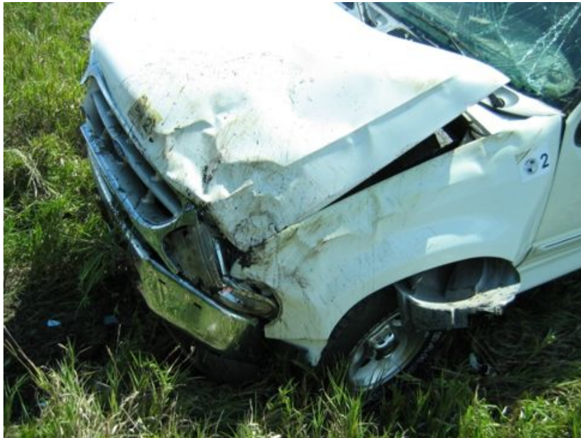
Circular Scratches indicate rotation
