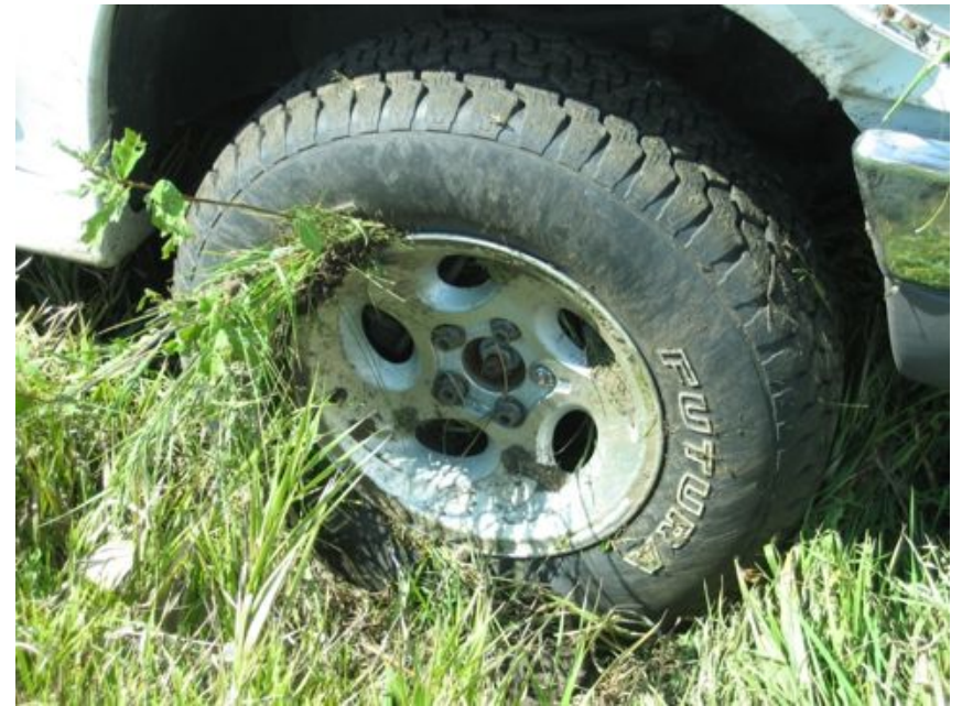
Grass Trapped between Tire and Rim
