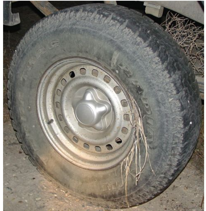
Grass Trapped between Tire and Rim
