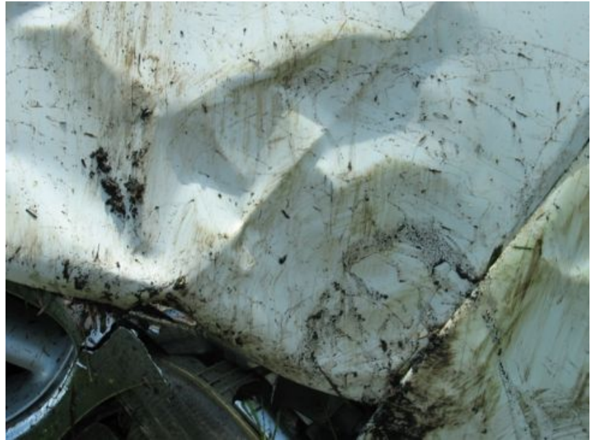
Circular Scratches indicate rotation
