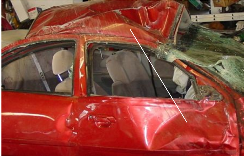
Lines show angle of scratches
