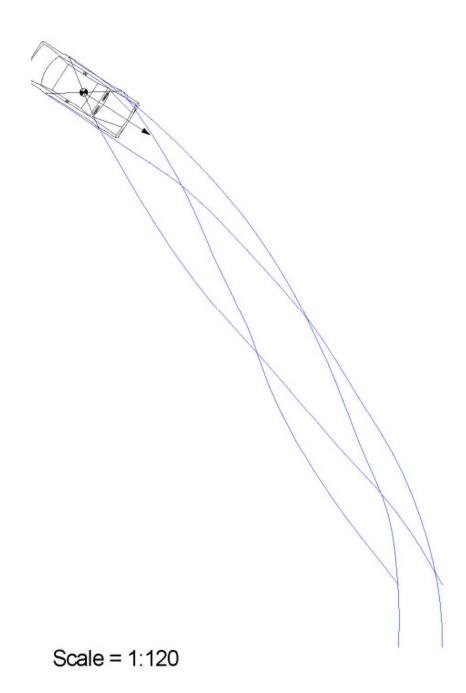
This vehicle has come to rest after impact, leaving the tire marks shown.
