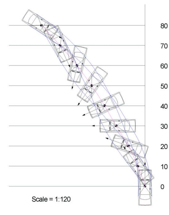
The heading of the vehicle is the direction in which the headlights are pointing.
